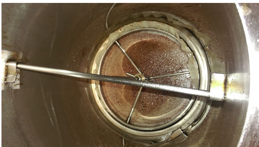
Figure 7 - The filter paper after one filtration run
