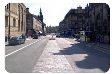
Visual Narrowing (material)- helps to narrow the road and reduce speeds
