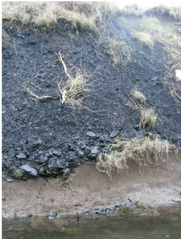
Photo GGS_3 P5: Made ground, consisting of loosely consolidated mudstone clasts, (likely to be waste material from local mining) overlying natural superficial deposits in a river bank section along the Lavern water (GGS_3b). Looking SE.
