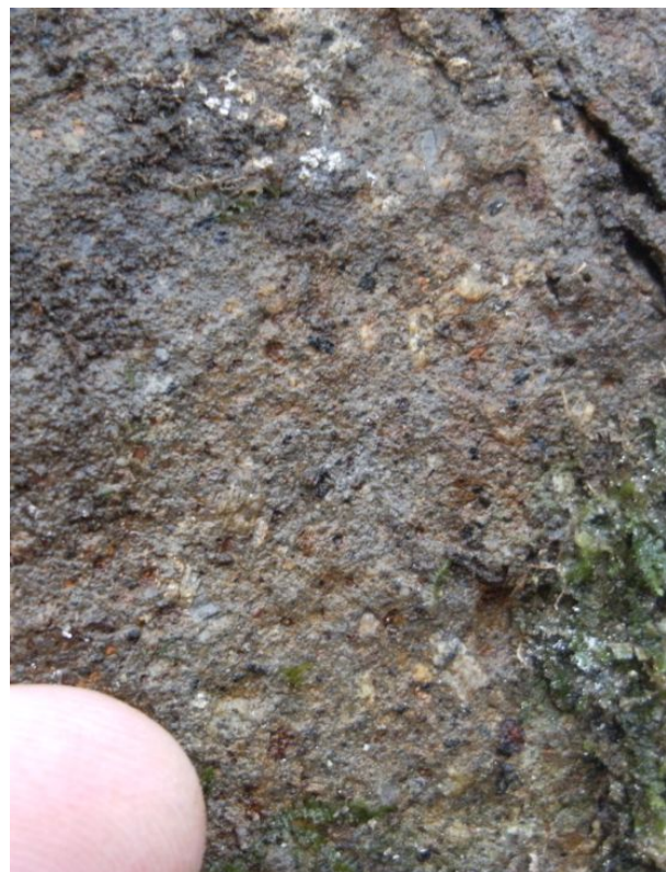
Photo GGS_1 P3: Close-up of the basaltic rock forming one of the lava flows seen in the quarry. The phenocrysts (large crystals) can be identified within a fine-grained groundmass.
