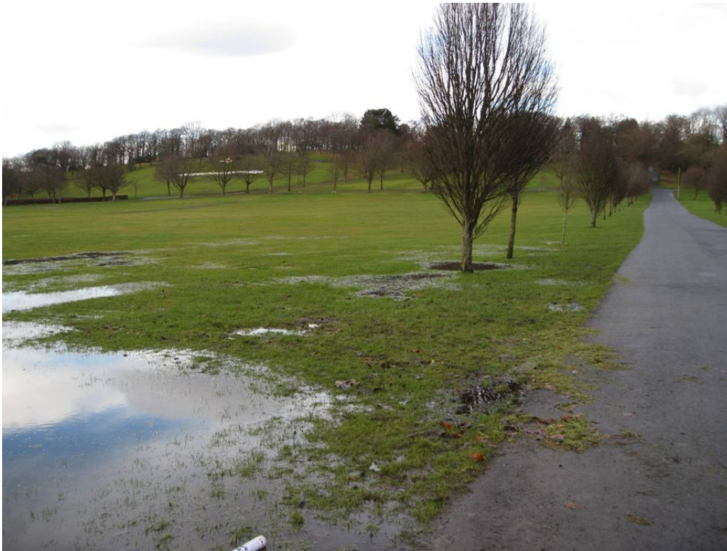
Photo GGS_18_P1: Bellahouston Park looking north towards the drumlin (hill topped with trees) from a flat inter-drumlin area underlain by raised glaciomarine sediments. The Glaciomarine clays have low permeability and the area in the bottom left is poorly drained after heavy rain.
