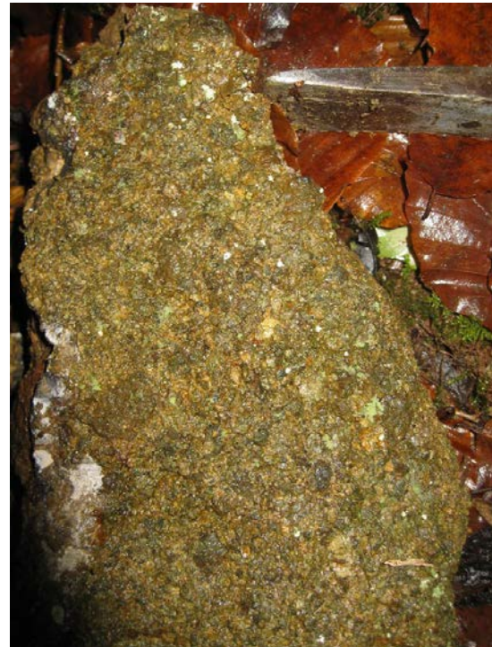
Photo GGS_2 P3: Close-up of an agglomerate bed, located in the lower part of the section. The individual grains of volcanic material (eroded from the Clyde Plateau Volcanic Formation) can be clearly seen.
