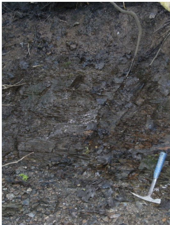
Photo GGS_3 P2: Sequence of well-jointed, thinly-bedded, dark-grey mudstones (GGS_3b). Looking SE.
