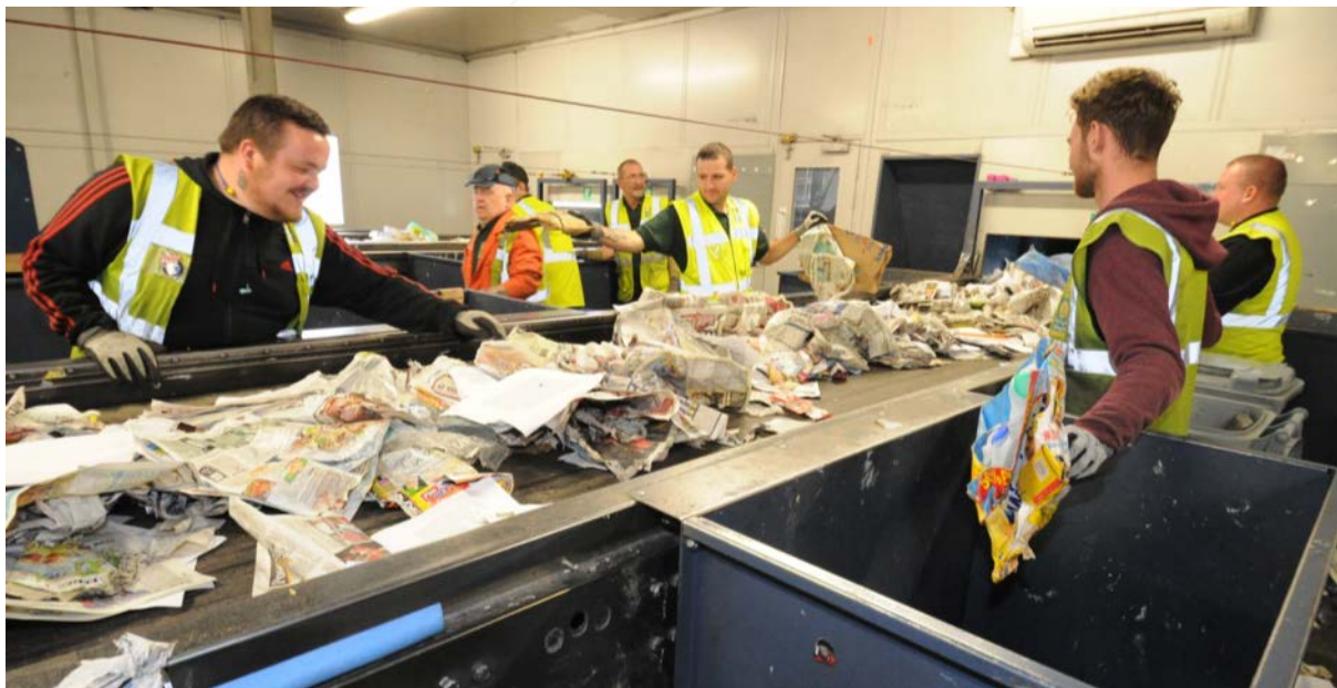
Manual waste separation at Blochairn MRF
